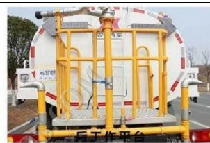
Back Working Platform
